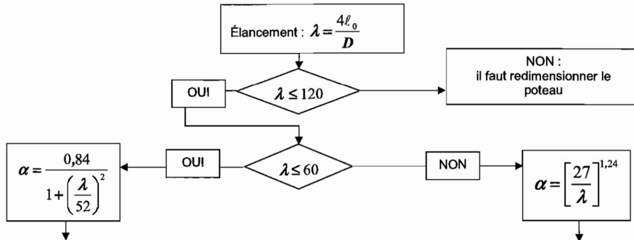
$$N_{Ed} \leq N_{Rd} \quad \text{et} \quad N_{Rd} = \alpha k_h [A_c f_{cd} + A_s f_{yd}] \quad \text{ou} \quad N_{Rd} = \alpha k_h A_c [f_{cd} + \rho f_{yd}]$$
